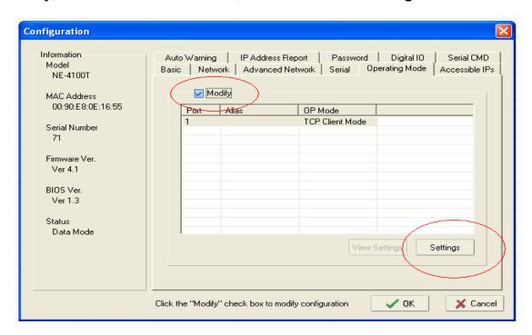
Select **TCP Client Mode** in the **Operating Mode** box. A maximum of four destination IPs can be entered in the **Destination Host** section.
