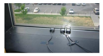
Figure 1: Antenna placement inside window
