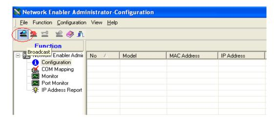
1. The Broadcast Search window will open and display the Model, IP Address, MAC Address, and Progress of the search for that particular device.
