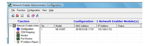
In this section, we illustrate how to access the NE-4100T's configuration utility. You should first make sure that you can connect over the network from your computer to the NE-4100T.
