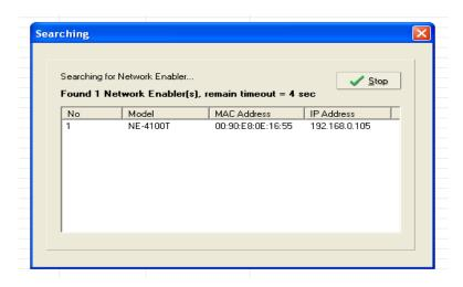
2. When the search is complete, the Broadcast Search window will close, and the NE-4100Ts that were located will be displayed in the right pane of the Administrator window. If you found more than one device connected to this network, refer to the MAC address sticker on your device(s) to determine which device(s) are the ones you wish to configure. To configure an NE-4100T, place the cursor over the row displaying that NE-4100T's information, and then double-click the left mouse button.
