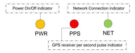
Figure 4: Indication LEDs
